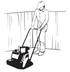
Step 3 Add Sand or Free Drainage Material\* to Base, Compact and Level with a Straight Edge
